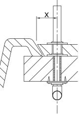
\* Indicates items to be supplied by installer. X= Distance from centerline of spout inlet to front of spout base plus 1/2" (13 mm).
